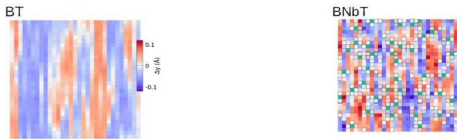
Figure 2: Molecular dynamics simulation of local displacements of B-site cations in \text{BaTiO}_3 (BT) and BNbT above the Curie temperature. Green squares indicate cation vacancies and black edges indicate Nb sites (Courtesy of M. Pasciak, Institute of Physics, Czech Academy of Sciences).
